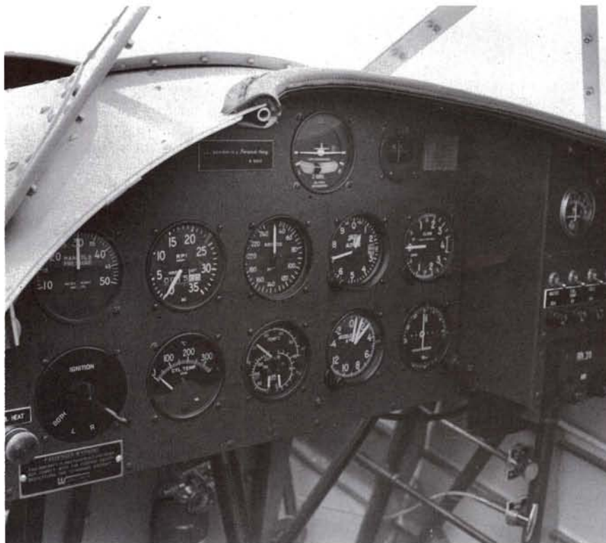
The rear cockpit instrument panel. Electrical panel is at right. Both cockpits are easily accessible through downward opening doors on left side.
