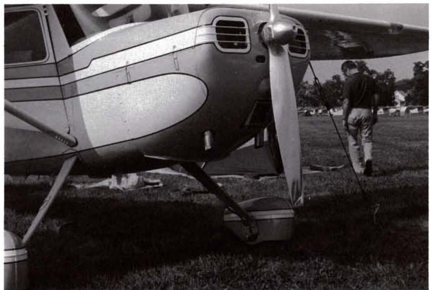
Original wheelpants were a $69 option in 1949! Note Brackett air filter on carb intake. Just above is small clearance dome for vacuum pump. Skullcap spinner replaced "150" spinner which fatigued. Landing light in wing was rescued from a salvaged 182.
