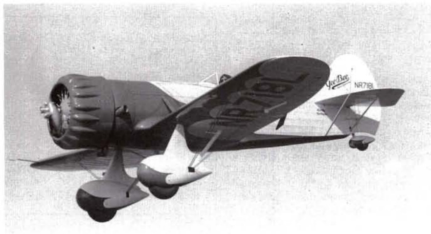
The aileron mass balance is visible in this view.
