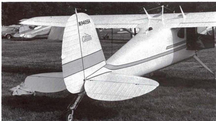
Tail view shows Scott 3200 tailwheel mounted on leaf spring that uses a "170" main spring for added ruggedness. Note large trim surface on right elevator. Very small fixed trim is visible on rudder, just below navigation light.
