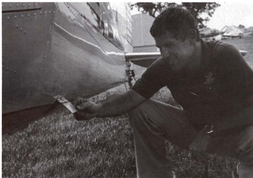
Jack Cronin demonstrates the spring-loaded door on the APU receptacle. From this plug, a 15 foot welding cable attaches to the car battery and he is ready for a jump start. APU plug is well away from engine and propeller area for safety.
