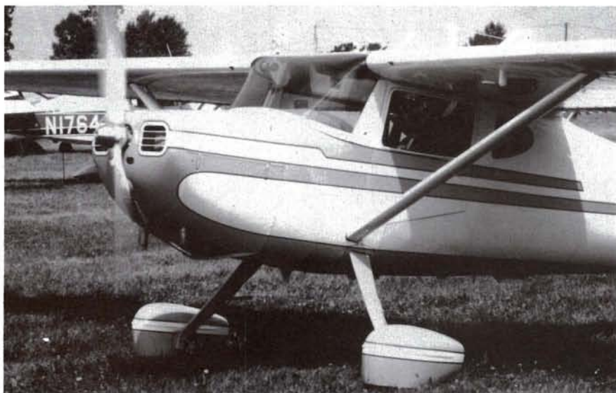
Jack Cronin taxis his 140A to the active runway at Oshkosh '84. Note heated pitot below left wing. Standard pitot extended from leading edge of left wing.
