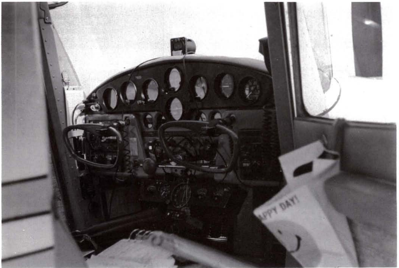
A look inside reveals full custom IFR panel that was undreamed of when Cessna built this plane in 1949! Jack uses ADF and Loran extensively in the mountains as VHF can suffer terrain problems. Note arm rest on door. Custom interior is in complimentary colors.
